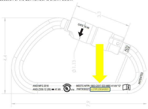
CMC requests that you inspect all carabiners from the lot number identified to ensure that the auto lock gate is not cracked. If the gate is cracked, immediately remove the unit from service and contact our customer support for resolution. You can contact customer support by calling (800) 513-7455 or (805) 562-9120, or via email at <a href="mailto:info@cmcpro.com">info@cmcpro.com</a>.
