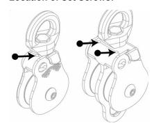
PLEASE NOTE: ProSwivel pulleys prior to 2018 were made in a slightly different manner than models made after 2018. Please refer to the corresponding section when inspecting your pulleys.
