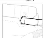
**Step 6:** Re-attach the airline fitting using the U-clip and the retaining screw. Tighten the retaining screw snug using the 3/32" hex Allen wrench.
