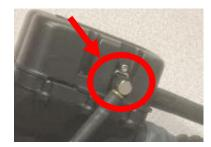
Use a spray bottle of soapy (dish detergent) water and spray the Auto Filter Cover airline fitting. Look for bubbles for 30 seconds — There should be no signs of visible bubbles that would indicate an air leak from this fitting (No bubbles = leak tight).
